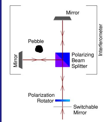
A horizontally polarised photon is sent into the device via the switchable mirror at the bottom. This mirror is timed to make the photon go through the system N times.
